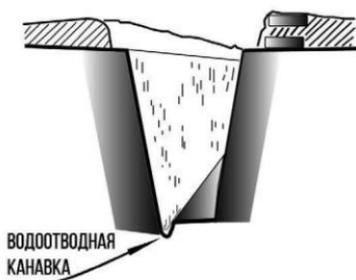
Figure 2. Drainage groove at the bottom of the trench
